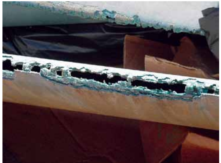
Figure 7: Severely Eroded Fan Blades
